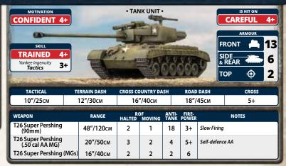
The men of the 3<sup>rd</sup> Armored Division's maintenance workshops further modified the tank by cutting out armour plates from German Panther tanks and welding them to it, creating the unique T26E1-1 'Super Pershing'.
