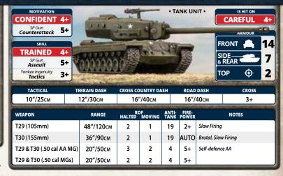
The T30 shares many of the features of the T29, but is armed with the even larger 155mm gun. It too has two-part ammunition and comes with an additional loader. The 155mm gun does not have the range of the 105mm gun, but is more destructive once it penetrates an enemy vehicle.
