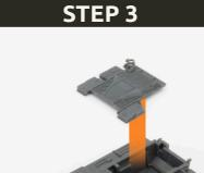
Attach the engine deck to the top of the hull.
